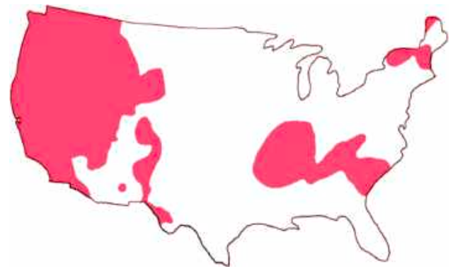
Fig. 5. Approximate mapping of the zones in which current seismic codes do not allow the construction of URM buildings in the United States [15].
