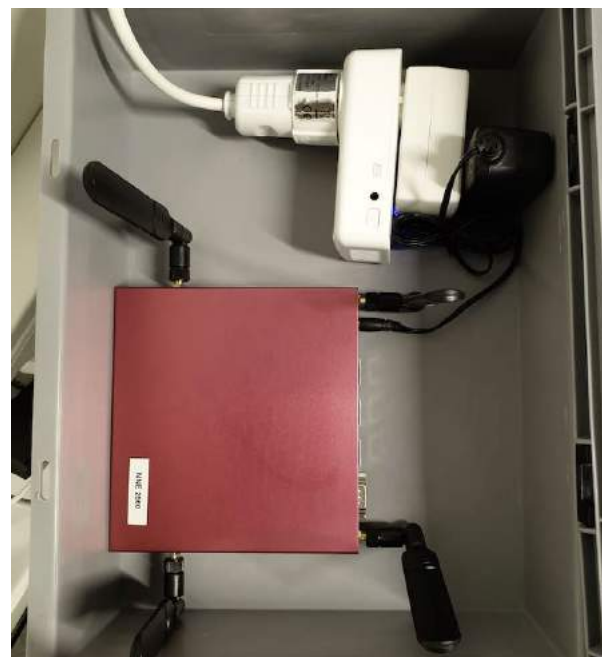
FIGURE 1. Measurement node. The red box encloses the single board computer. The box also includes a smart power socket that can be rebooted via SMS.
