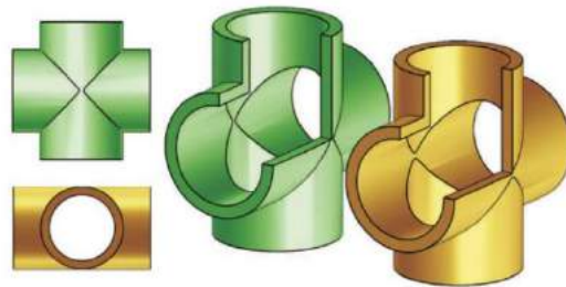
Figure 4.2: Pipes meeting at a right angle (Glaeser, 2007)
